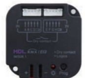
8 Zone Dry Contact Module
