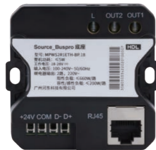
Source-Buspro Power Interface
